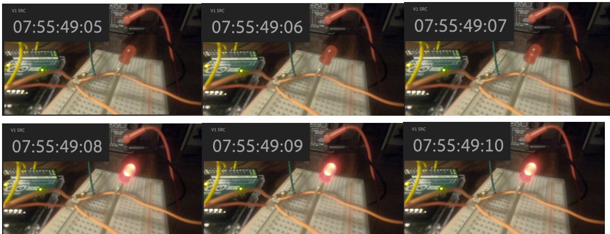
Figure 8. Frame by frame images taken from the GoPro of the Arduino when its LED turns on. The corresponding LTC timecodes jammed by the SyncBac into the GoPro are shown in the upper left of each frame. We can observe that these timecodes
